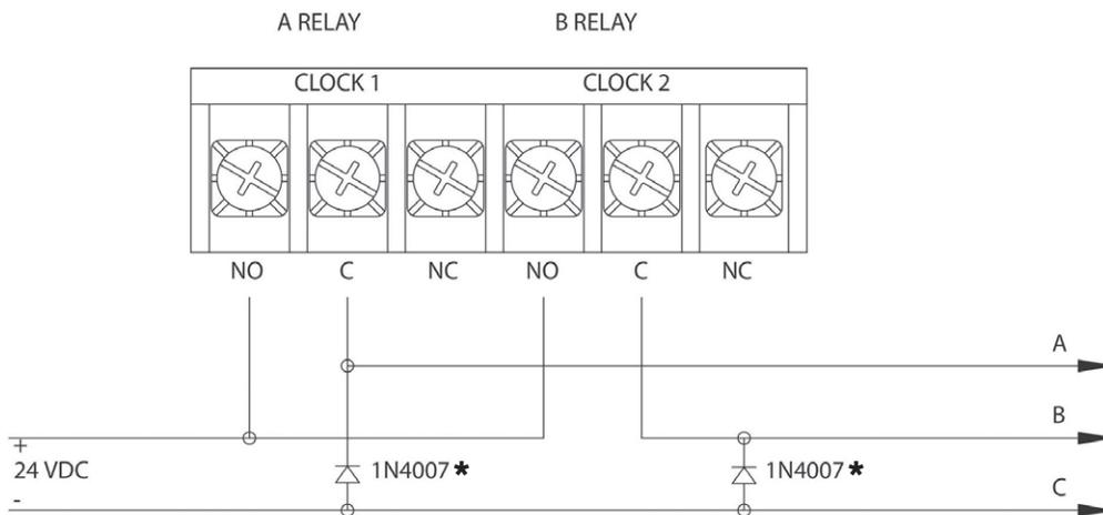
**\*Rectifier diodes recommended for relay protection.**
