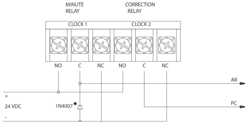
\*Rectifier diode recommended for proper operation of reversing polarity.
