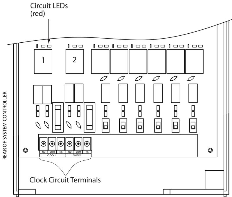
See Appendix I on Page 63 for Clock Circuit Wiring Diagram
