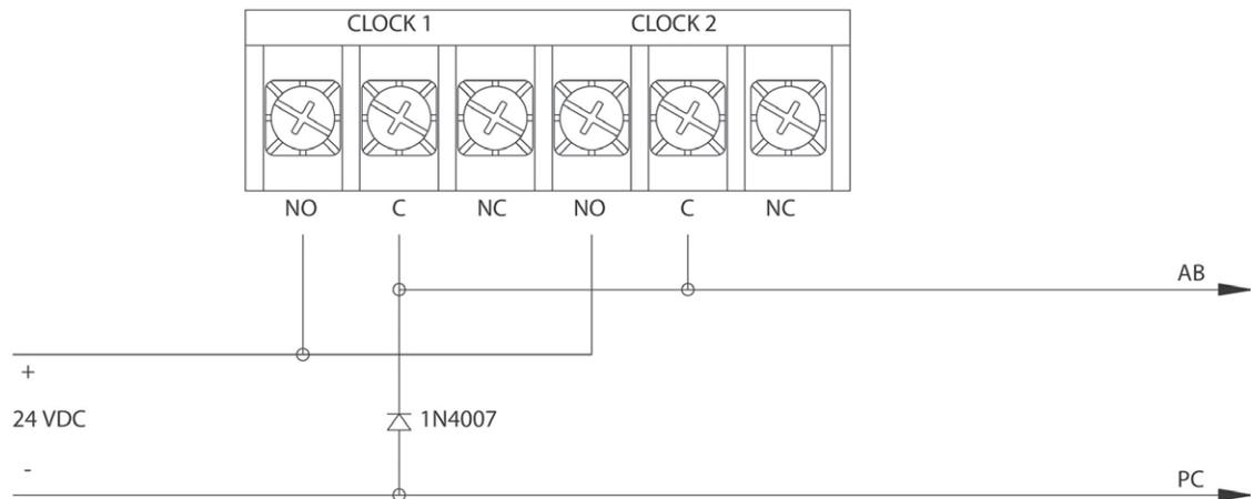
Clock Code 38 - 2 wire Reverse Polarity Minute Impulse (59th minute) with 12hr Correction
