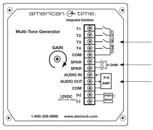
Apply a contact closure from T1, T2, T3 or T4 to C from a time switch, master clock or push button control. Apply jumpers to the T1, T2, T3 or T4 terminals as required for additional tones. See the Tone Selection Table below.
