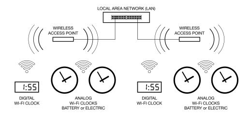
Each Wi-Fi clock can be factory-configured to receive the precise time signal from your network server. They also automatically correct for the Daylight Saving Time changes and require little maintenance. Wi-Fi clocks only require synchronization twice per day using SNTP and create very little network traffic with staggered wake times. The electric and digital models can be user-selected to synchronize at a desired frequency.
