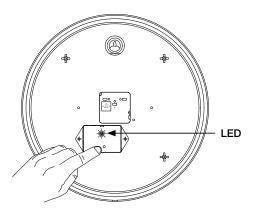
Each operation is proceeded by a number of orange flashes. If the button is released after the operational flash count (see list below) it will attempt the specific operation listed.
