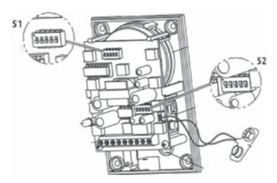
The table below shows the different alarm volumes and timing available and the proper dip switch setting for each.
