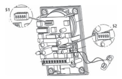
The table below shows the different alarm tones available and the proper dip switch setting for each.
