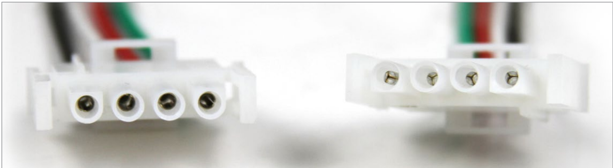
Female pin connection to wall. Cut this end if necessary.
