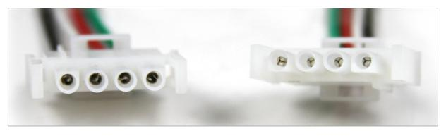
Female pin connection to wall. **Cut this end if necessary.**
