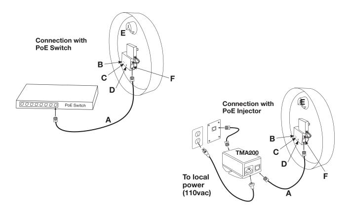
A=PoE connection (CAT 5 or higher Ethernet patch cable–included) B=Status LED C=Relay LED D=Default Button E=Keyhole Hanger F=PoE Receiver
