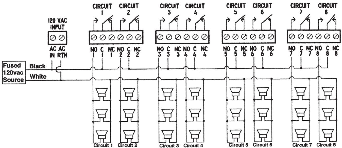
This diagram is using 120vac bells (user supplied step-down transformer required for low voltage (24vac) signals).
